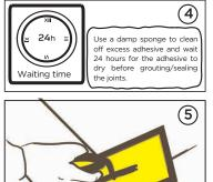
Grout and seal the joints using a Weber rubber trowel. Wait 24 hours before use
